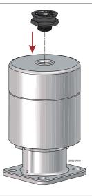
(2) Fit the sensor target to the actuator stem.
