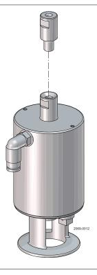
2 Mount the adapter to the actuator using 3 hex applying a moment of 1..1.5 Nm.
