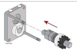
Slide auxiliary shaft (22), with gear, in to position in the back plate (2). Both ends of the shaft are identical.
