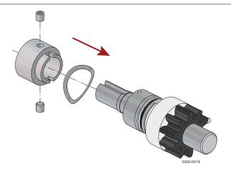
(5) Gently move the spring retainer back, releaseing the spring pressure until the gap between the spring retainer and rotary seal ring is 1.5mm (0,059").
