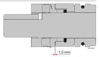
6 Tighten retaining screws (13) equally and gradually until hand tight.
