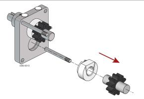
**6** Remove the drive shaft assembly (19) complete with the rear bush (9), gear (20) and seal assembly. **NOTE**: The back plate (2) can remian fixed to the motor (or other mounting as applicable) whilst dismantling is carried out.
