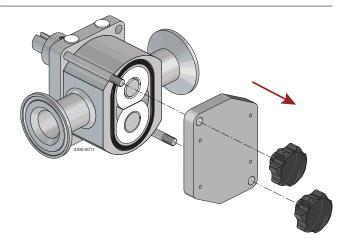
(4) Remove body (1) together with the Front and Rear body O-rings (5). **NOTE**: Front bushes (4) may stay in the body but can be removed by pushing out.
