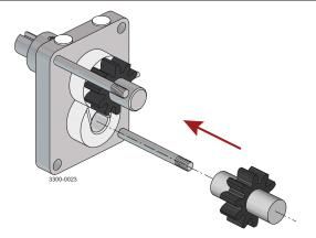
(4) Fit 1 of the O-rings (5) to the back of the body (1). The ports are offset from the centerline of the body, with the narrowest width towards the back (as shown).
