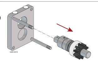
7 Loosen the seal retaining screws (13) and remove the seal assembly and rear bush (9) from the drive shaft.
