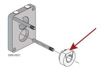
2 Press, by hand, the drive shaft assembly into (through) the bore in the back plate (2) untill fully seated, making sure the flat sides of the bushes are aligned.
