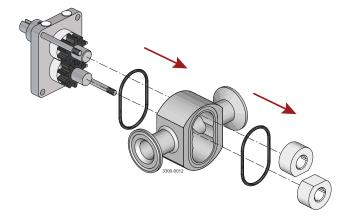
(5) Remove the auxiliary shaft (22) with gear (20) and the rear bush (9) from the back plate (2).
