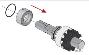
4 Fit wave spring (14) on to spring retainer (12), then slide the spring retainer on to the shaft ensuring to align the pins in the rotary seal with the slots in the spring retainer fully until the seal faces meet and the spring is fully compressed.
