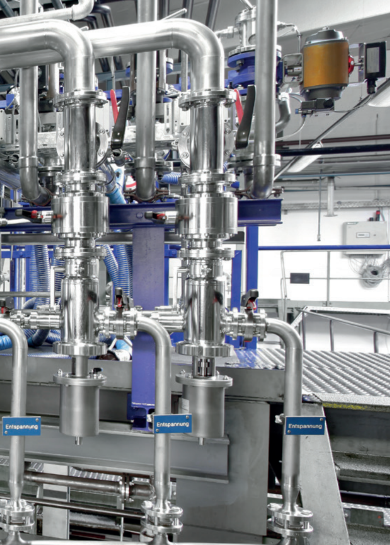
Pigging systems in lubricant production
