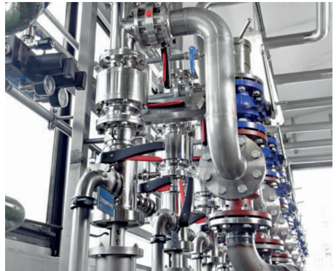
Pigging systems in lubricant production
