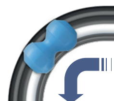
Pigging of DIN bends without product mixing
